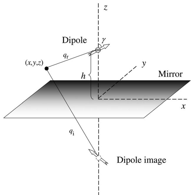
Fig. 1. We use an  $xyz$  coordinate system as shown in the diagram. The distance between the source and the observation point is indicated by  $q_r$ , and  $q_i$  is the distance between the observation point and the mirror dipole.
