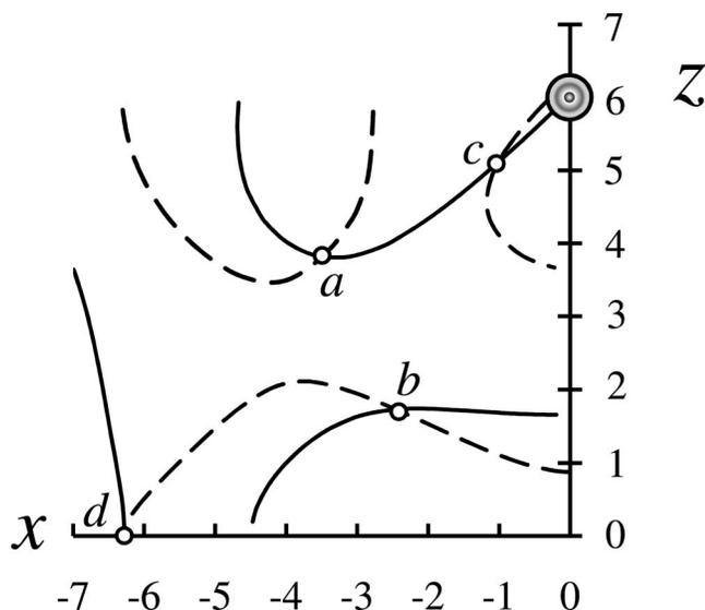
Fig. 3. The solid (dashed) curves represent the solutions of  $\text{Re } B_y = 0$  ( $\text{Im } B_y = 0$ ) in the  $xz$  plane. At the intersections we have  $B_y = 0$ , and therefore  $\mathbf{B} = 0$  and  $\mathbf{S} = 0$ .
