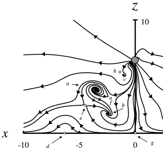
Fig. 2. Field line pattern in the  $xz$  plane for radiation emitted by a dipole oscillating under an angle of  $\gamma=\pi/4$  with the  $z$  axis and located a distance of  $h=2\pi$  above the interface.
