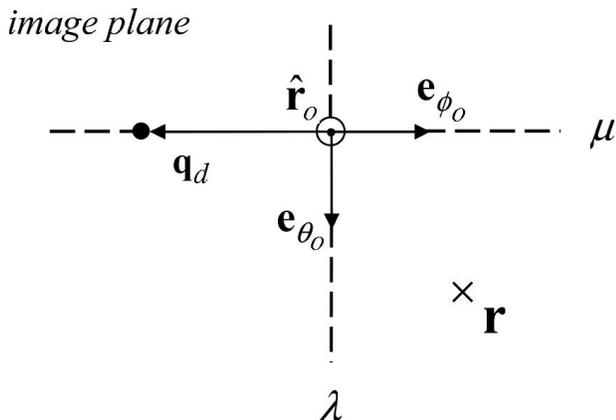
Fig. 2. Image plane in the observation direction  $(\theta_o, \phi_o)$  is perpendicular to the radial unit vector  $\hat{\mathbf{r}}_o$ . The Cartesian coordinates  $(\lambda, \mu)$  in this plane are defined as shown. The field line of the Poynting vector that runs into this direction intersects the image plane at the point indicated by the displacement vector  $\mathbf{q}_d$ , which is along the  $\mu$  axis (and is in the direction shown for  $\tau = 1$ ).
