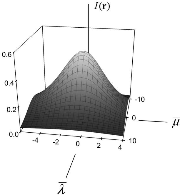
Fig. 3. Shown is the intensity distribution  $I(\mathbf{r})$  in the  $\bar{\lambda}\bar{\mu}$  plane for  $\theta_o = \pi/2$  and  $\tau = 1$ . The peak of the distribution is at the negative side of the  $\bar{\mu}$  axis, and this is a result of the spiraling of the field lines in the counterclockwise direction near the position of the dipole.
